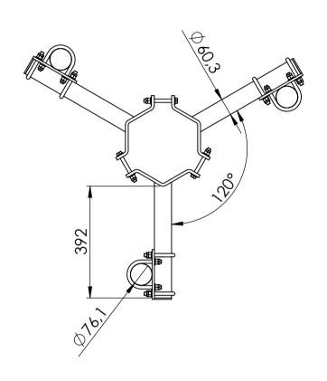
Basic wind Vb,0 = 27 m/s Terrain class TC = 1 Max height of installation = 70m
