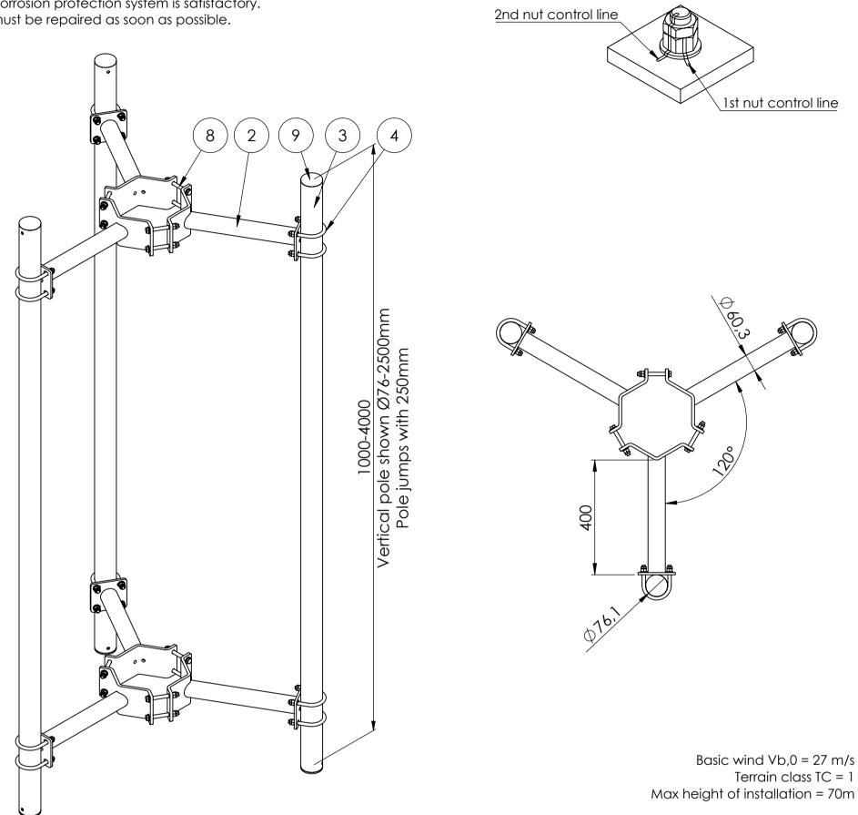
Max loads per 1 mount pole from equipment: 150kg, CxA=1.6m2
