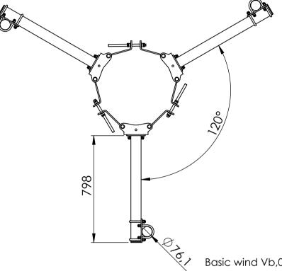
Basic wind Vb,0 = 27 m/sTerrain class TC = 1 Max height of installation = 70m
