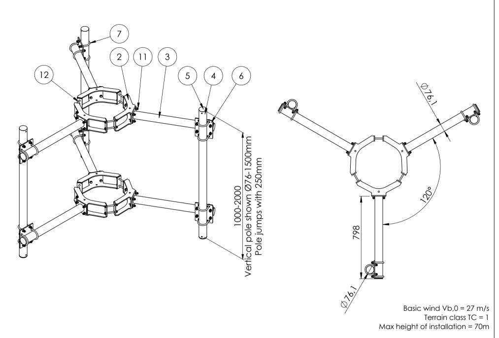
Max loads per 1 mount pole from equipment: 100kg, CxA=1.0m2
