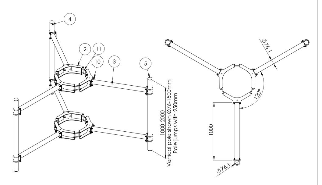
Basic wind Vb,0 = 27 m/s Terrain class TC = 1 Max height of installation = 70m
