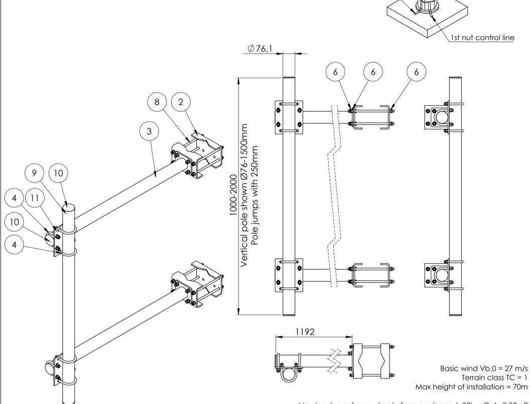
Max loads per 1 mount pole from equipment: 33kg, CxA=0.33m2
